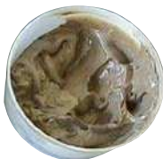
Used grease: colour turned greyish
