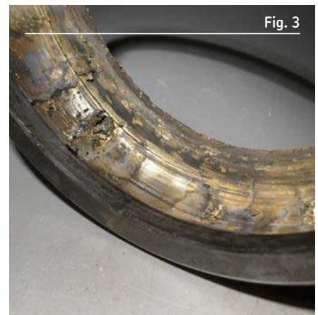
Loss of internal radial clearance leading to a seized bearing
